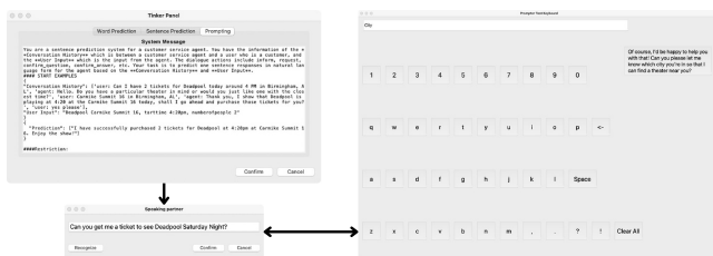
Figure 4: The test virtual keyboard for the prompt produced from Promptor . This keyboard offers designers firsthand experience of a GPT-empowered intelligent text entry system.
